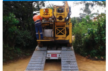
2.5M WIDE STEP DECK EASES UNLOADING
