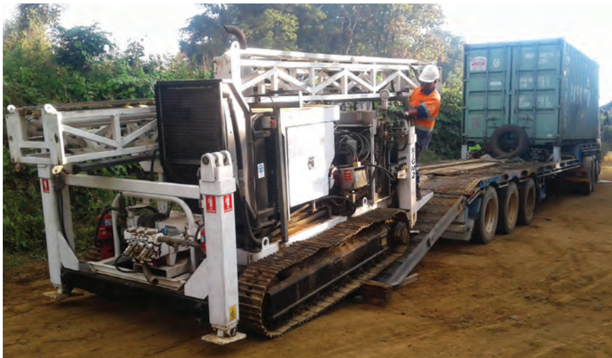
CEA MULTI-CARGO STEP DECK TRAILER UNLOADING DRILL RIG AND CONTAINER
