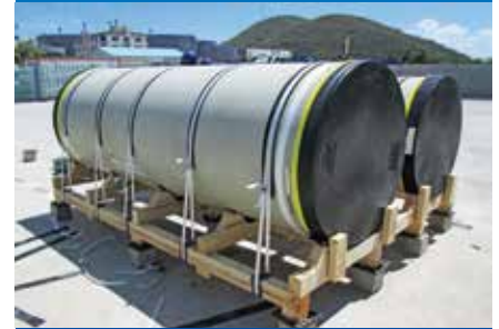
GAS SPOOLS STRAPPED TO PACKING FRAME
