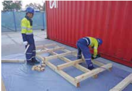
PACKING FRAMES BEING FABRICATED
