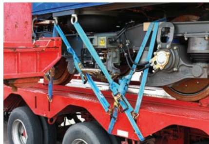
CARRIAGES SECURED WITH RATCHET STRAPS
