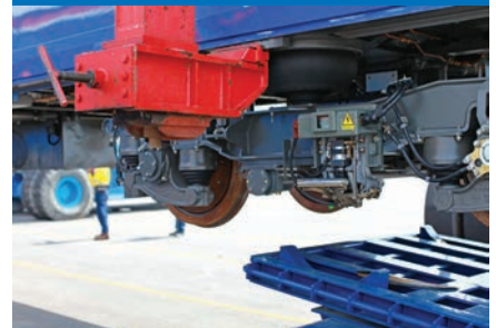
CARRIAGE LIFTED FROM ITS BOGIE
