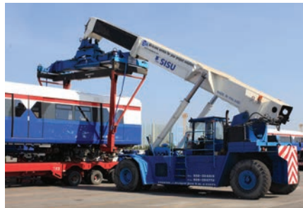
SPECIALISED LIFTING CLAMPS ATTACHED
