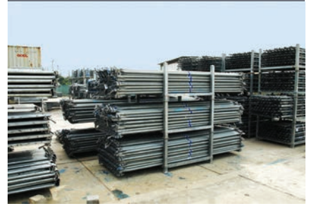
SCAFFOLDING PIECES SECURED ON RACKS
