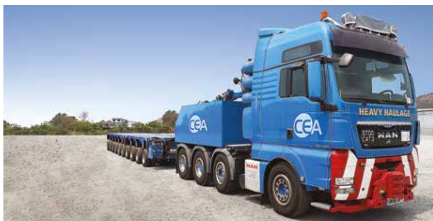
FLAGSHIP OF THE CEA FLEET THE MAN TGX 680 PRIME MOVER WITH HYDRAULIC TRAILER
