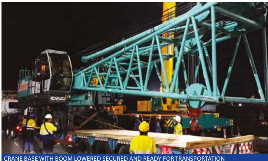
CRANE BASE WITH BOOM LOWERED SECURED AND READY FOR TRANSPORTATION
