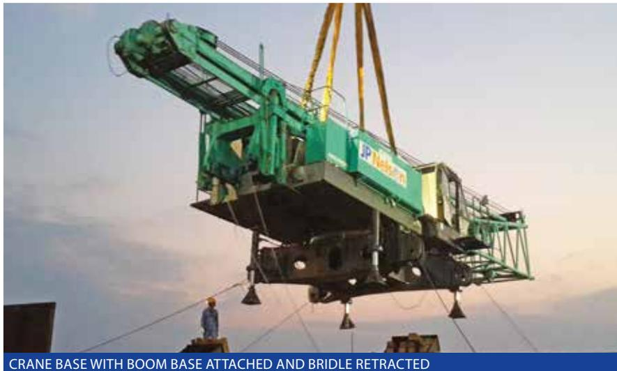
CRANE BASE WITH BOOM BASE ATTACHED AND BRIDLE RETRACTED
