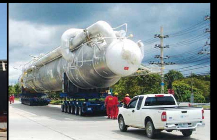
Transporting cryo-genic column for gas separation plant
