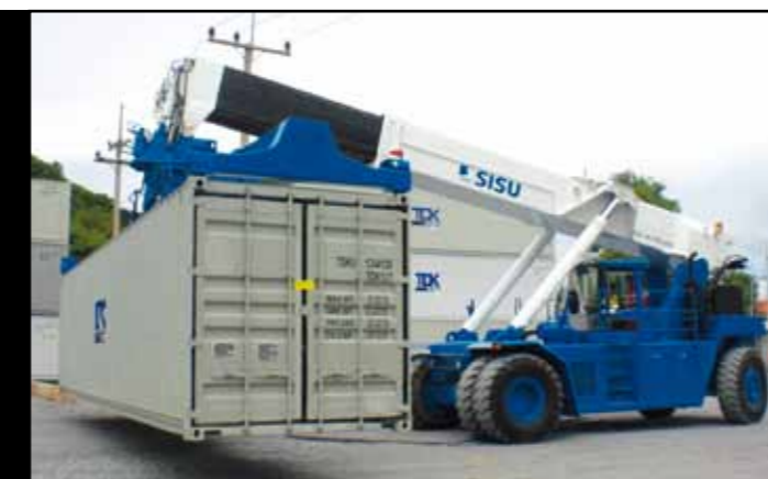
Loading of containers using 45t reach stacker
