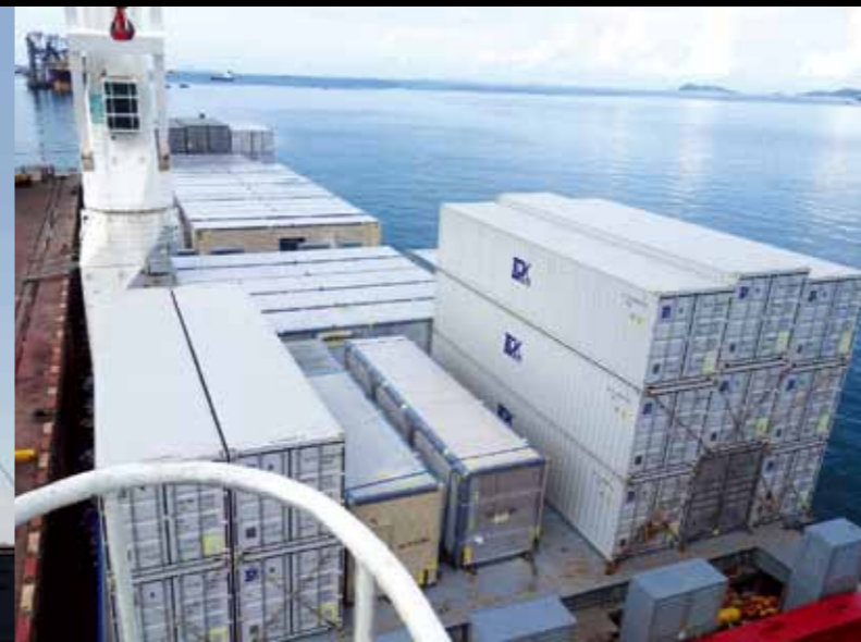
Modules loaded and lashed prior to sail away
