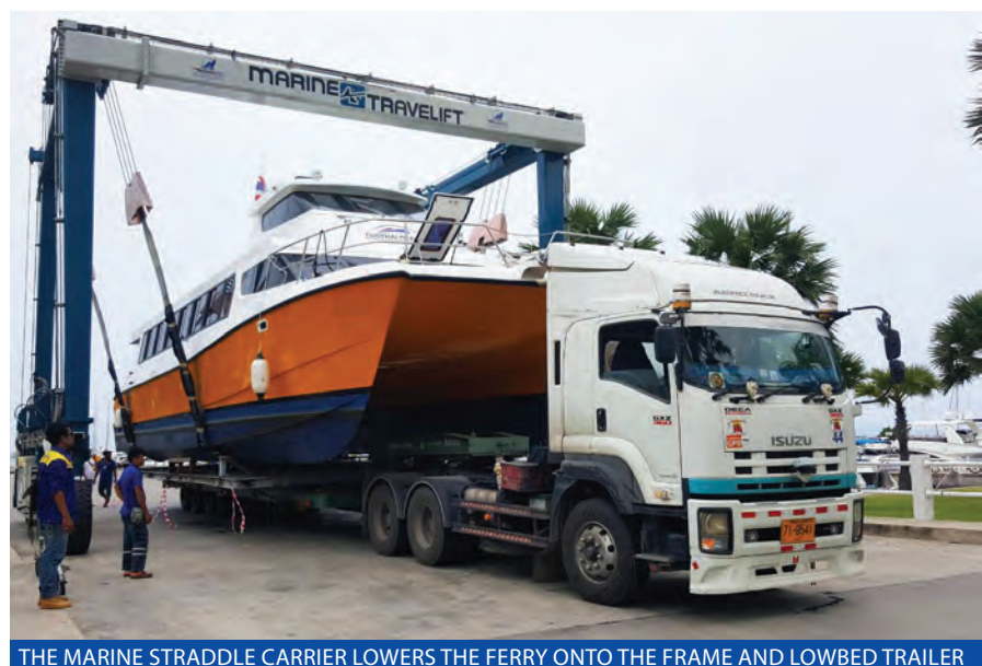
THE MARINE STRADDLE CARRIER LOWERS THE FERRY ONTO THE FRAME AND LOWBED TRAILER
