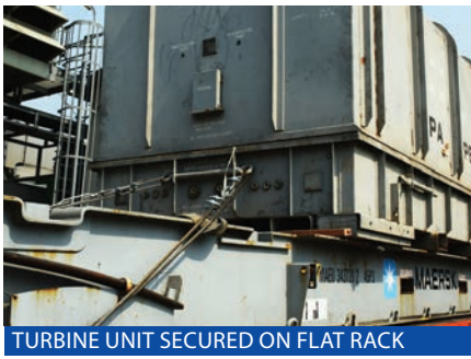
TURBINE UNIT SECURED ON FLAT RACK
