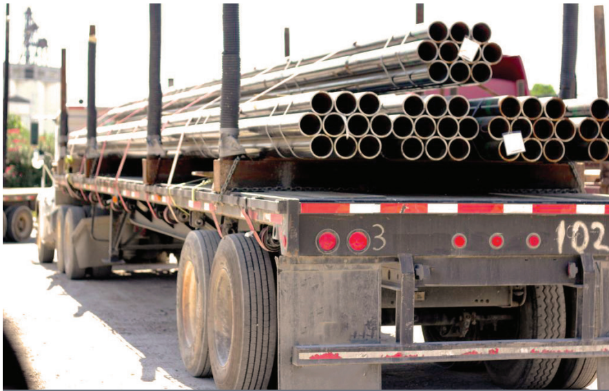
DRILL PIPE LASHED AND SECURED READY FOR TRANSPORTATION
