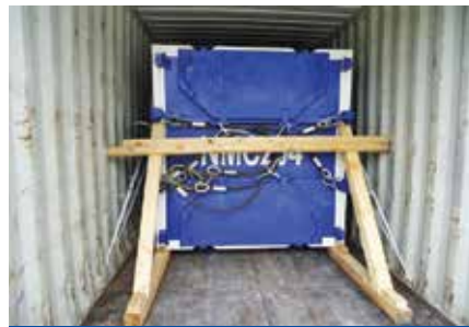
WOODEN STOPPERS INSTALLED
