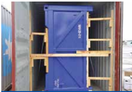
WOODEN CHOCKS INSTALLED
