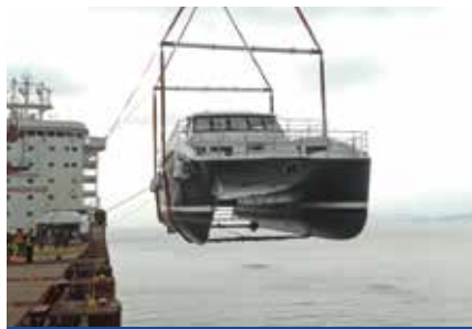
CRANE LIFTS THE BOAT ON TO THE TOP DECK
