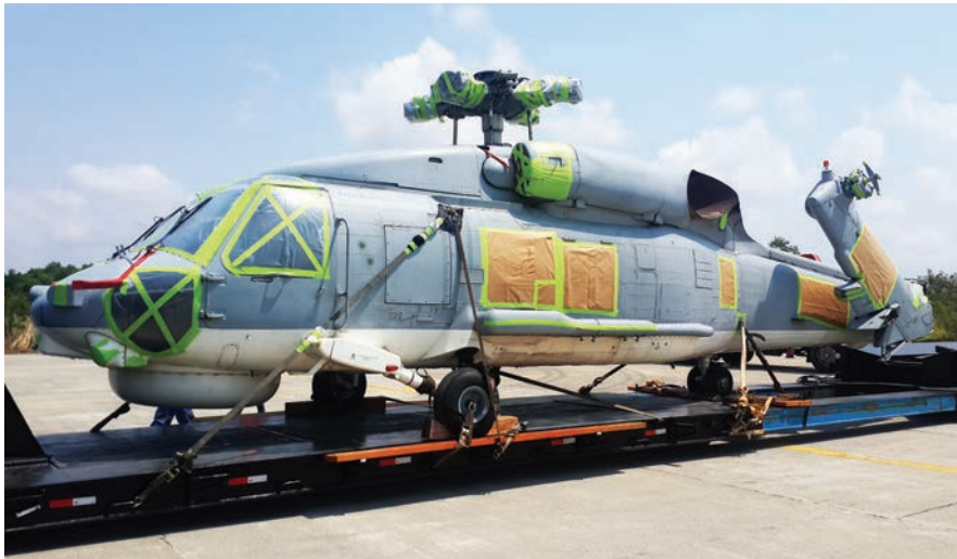
SEAHAWK STRAPPED & SECURED ON A DROP-DECK AIR RIDE TRAILER READY TO LEAVE UTAPAO
