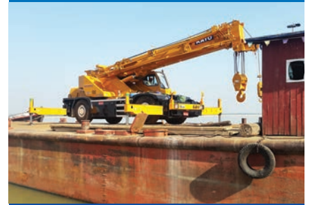
CEA 70 T CRANE TRANSPORTED BY BARGE
