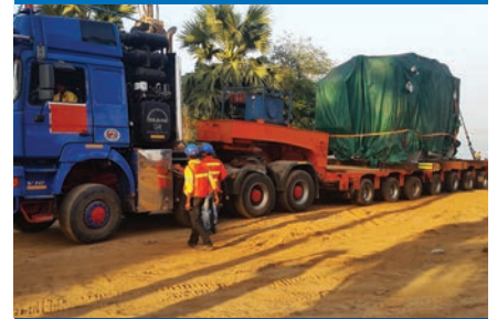
TRANSFORMER ON A MULTI AXLE TRAILER
